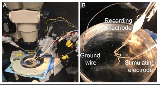
**Figure 10:** Set up to record compound action potentials from the sciatic nerve. (A) The recording dish filled with normal Ringer and the two electrodes with micromanipulators. (B) The recording and stimulating electrodes in place with Vaseline plugs around the nerve and the lumen of the electrodes. A ground wire is attached to the Faraday cage around the recording set up.
